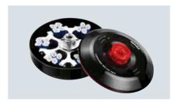
Aerosol-tight Eppendorf QuickLock swingbucket rotor for 24 x 1.5/2.0 mL tubes spins up to 16,050 x g/12,700 rpm. Swing-bucket design is ideal for phase separation or to collect pellets at the bottom of the tube (S-24-11-AT; Cat. No. 5409715003).
