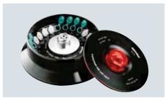
Aerosol-tight Eppendorf QuickLock Kit rotor for 24 x spin columns and 1.5/2.0 mL tubes. Designed with an extra high rim to support open tube lids during centrifugation. Spins at max. 19,100 x g/13,200 rpm (FA-45-24-11-Kit; Catalog No. 5409704001).
