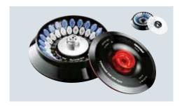
Aerosol-tight Eppendorf QuickLock rotor for 48 x 1.5/2.0 mL tubes provides speed up to 18,210 x g/12,700 rpm (FA-45-48-11; Catalog No. 5409710001). Also available with basic plastic lid (F-45-48-11; Catalog No. 5409712004).
