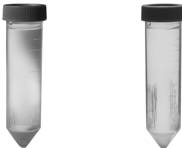
Figure 8. Examples of Tubes with Minimum and Moderate Crazing
