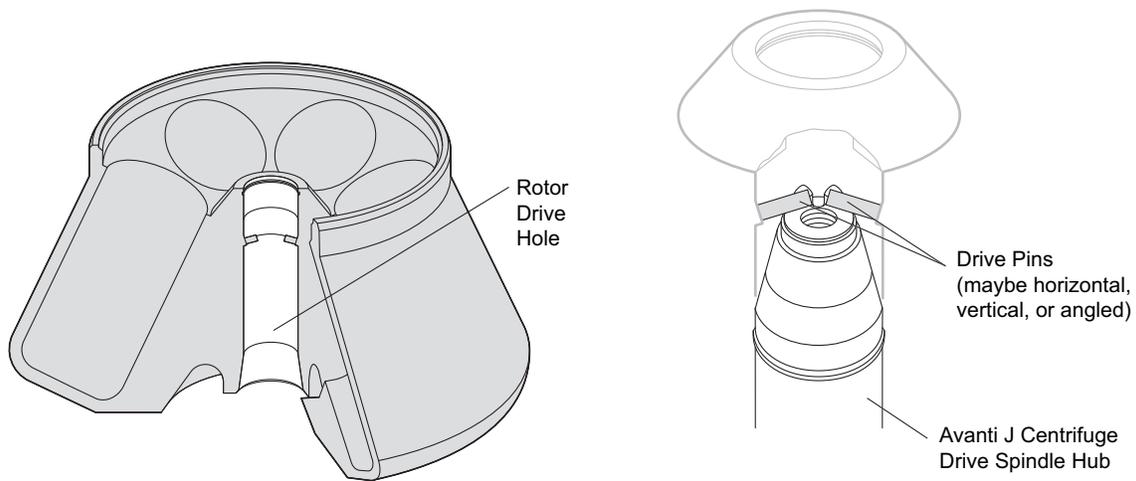
Figure 2. Rotor Drive Pin Location and Orientation
