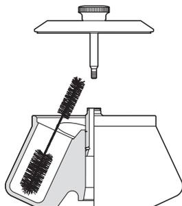
3. Thoroughly rinse the cleaned rotor and components with distilled water.
