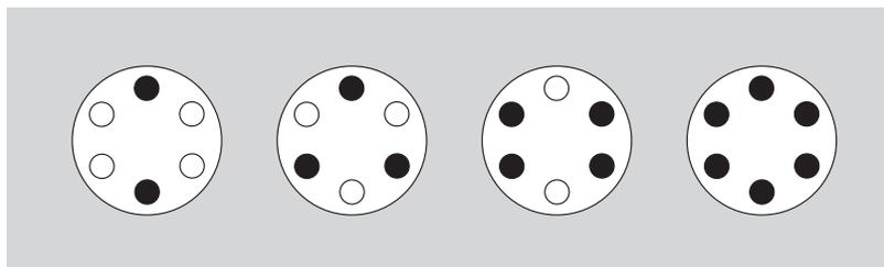
Figure 1. Arranging Tubes or Bottles in the Rotor.
