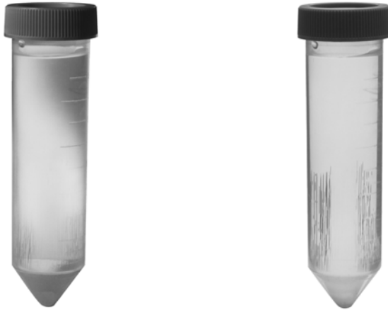
Figure 10 Examples of Tubes with Minimum and Moderate Crazing
