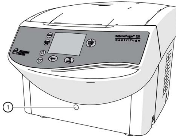
Figure 3.2 Removing the Emergency Access Plug
