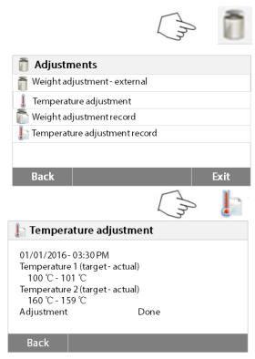
Press Weight and temperature adjustment button to access the adjustment screen.
