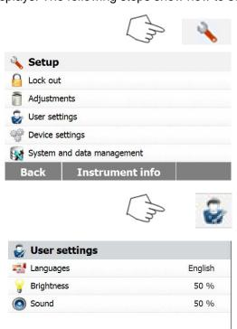
Press Setup button to access the Setup screen.
