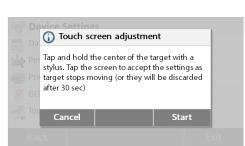
Press **Touch screen adjustment** to adjust the touch screen.
