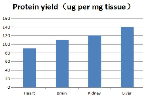
**Figure 1:** Protein yield with Tissue Protein Extraction Buffer. Tissue proteins were extracted from different mouse tissues using Tissue Protein Extraction Buffer protocol. The protein concentration of each lysate was estimated by BCA Protein Assay Kit.
