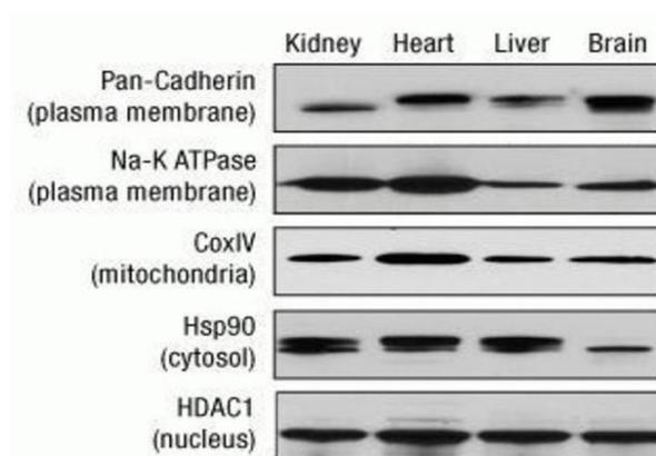
**Figure 2:** Protein identification, using Western Blot. The proteins were extracted from mouse tissues using Tissue Protein Extraction Buffer. Lysates (20µg) were separated by SDS-PAGE and transferred to a nitrocellulose membrane and probed using respective antibodies and chemiluminescent reagents.
