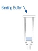
Note: It is also normal to add a small amount of imidazole (10 - 40 mM) to improve the selectivity of the binding of the histidine-tagged protein. It is important to use imidazole of high purity to avoid affecting O.D. 280 nm. It is also important to avoid inclusion of reagents such as EDTA or citrate.
