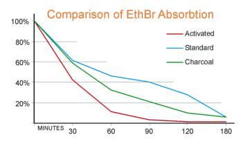
Typical comparative absorption of a 0.5ug/ml EtBr solution expressed as a % of the initial  $A_{285}$
